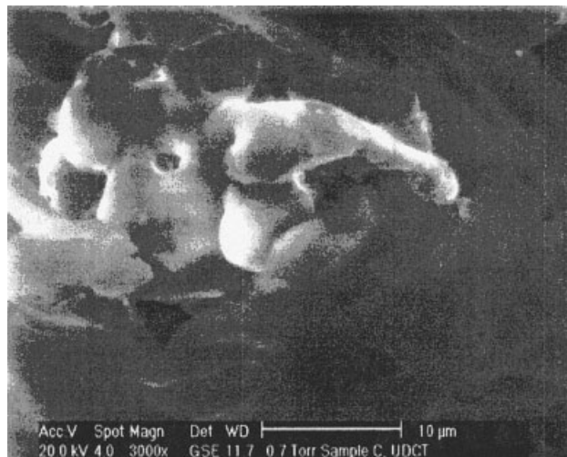
Figure 9 SEM micrograph of a fractured surface of treated 60 μ flyash/nylon 6 composite containing 30 wt % flyash.
